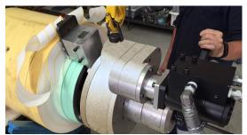
6" (152 mm) of polyethylene is removed from a steel pipe O.D. and beveled for welding spool pieces together.
