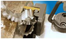
The EscoLock blade lock system and double threaded lock screw hold the blade securely in place to produce a thick chip that helps prolong blade life by transferring the heat to the chip and away from the Cutter Blade.
